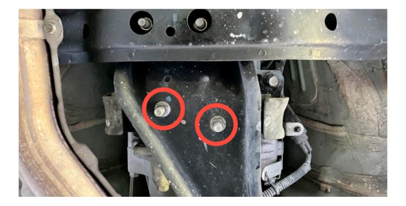
**STEP 9 -** Using a floor jack or pole jack, raise the transmission so that the rear cross member bolts can be reinstalled. Torque to 51.6 ft/lbs
