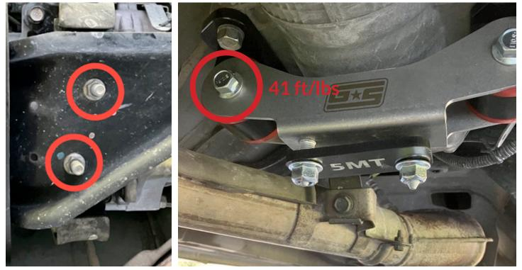
**STEP 8 -** Reinstall the transmission cradle, using the supplied 15mm nuts. Torque to 25.8 ft/lbs.
