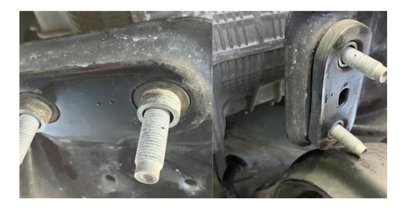
**STEP 11 -** Using your floor jack or pole jack, raise the transmission under the front cross member at the nuts that we just installed so that the 17mm cross member bolts can be installed fully. This ensures that we are not using the bolt to raise the transmission and possibly damaging the body threads. Torque to 103.3 ft/ lbs.
