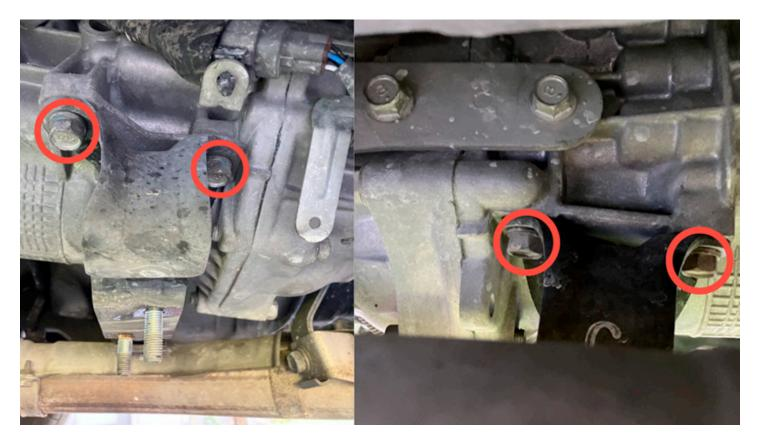
**STEP 6** - The two transmission mount bosses need to be removed from the GrimmSpeed mount bracket and installed first. The passenger side boss will only fit in one orientation, but it is possible to mount the driver's side boss backwards. Refer to the image below for the proper orientation. These bolts are 14mm bolts, torque these bolts to 25.8 ft/lbs.
