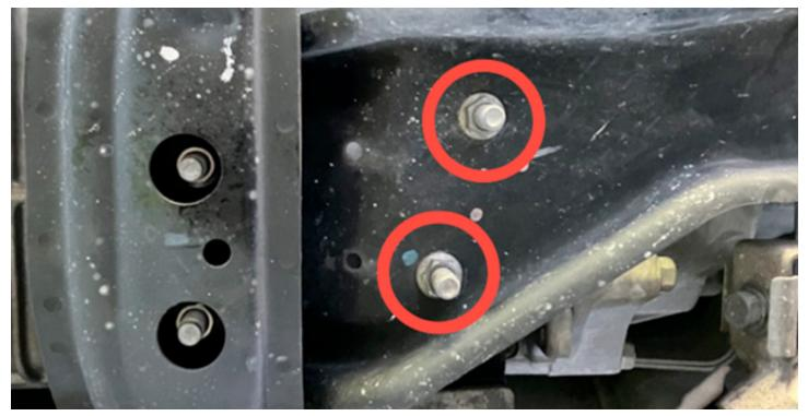
**STEP 5 -** With the transmission bracket out of the way, remove the four 14mm bolts holding the transmission mount to the transmission.
