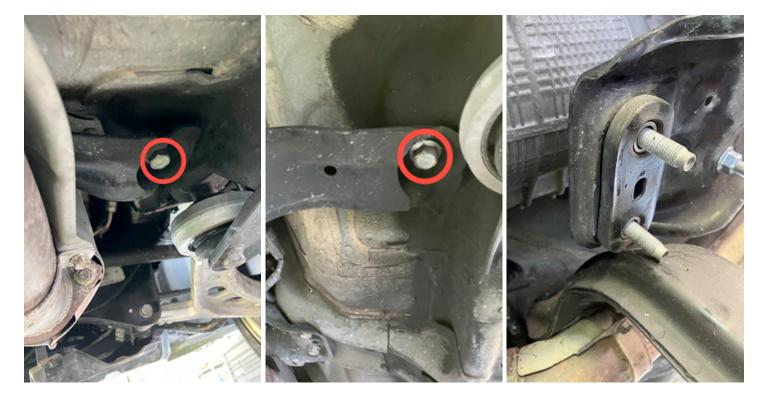
**STEP 3** - Using a 14 mm socket remove the two bolts holding the transmission mount to the rear cross member. Note the rubber isolator between the hardware bracket and the transmission cradle, it may fall off the cradle.
