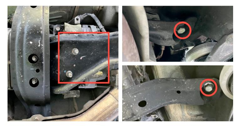
**STEP 12 -** Finally, torque the nuts securing the transmission cradle to the front cross member to 51.6 ft/lbs. Once these are tightened, you can lower your vehicle down and take it for a test drive!
