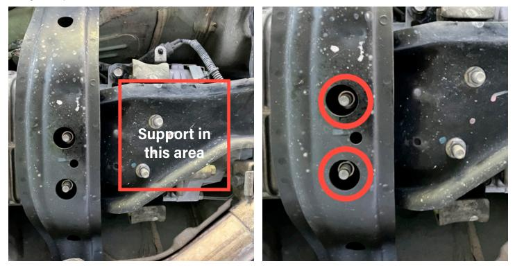
**STEP 2 -** Remove the two 17 mm bolts holding the front cross member to the body. You will them be able to slide the cross member over the exhaust and remove it. Note the rubber isolator between the cross member and transmission bracket.
