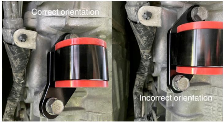
**STEP 7 -** Install the transmission mount bracket to the bosses. The bolts will only fit from front to rear of the car. The transmission mount bracket needs to be oriented so that the stud on the passenger's side is set forward. Using a 15mm box wrench and 15mm socket, torque to 41 lb-ft. If installing on a 5 speed transmission you will need to use the Transmission Mount 5MT adapter between the mount bracket and the transmission bracket.
