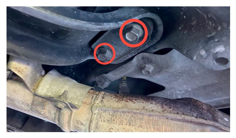
**STEP 10 -** Ensure that the front cross member stud bushings are seated properly in the transmission bracket. Install the isolator, and the front cross member to the transmission bracket. Only hand tighten these nuts for now.
