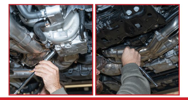
Carefully remove the three turbo studs with an E10 torx socket, taking care not to snap the studs. We highly recommended to use a ratchet instead of power tools to avoid snapping the studs. If you experience resistance, apply penetrating oil and consider heating the area around the studs. We recommend running an M10x1.25 tap through the threads in your turbo to ensure that there is no damage to the threads.
