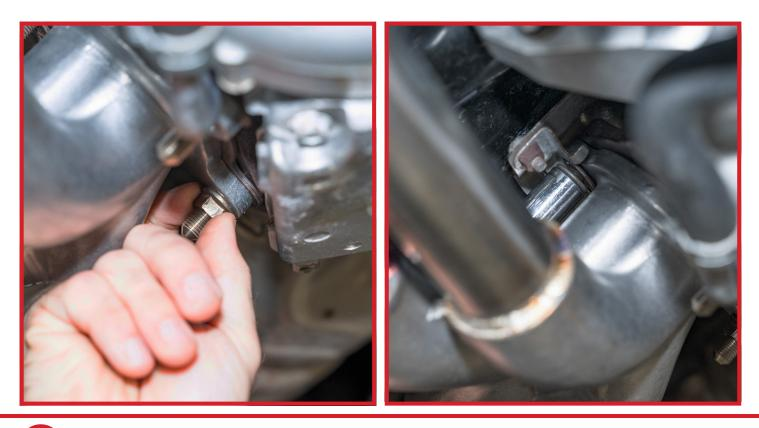
With the turbocharger secured to the new GrimmSpeed manifold, you can now fully torque down all six nuts attaching the header to the heads of the engine. These nuts will be torque to 47 ft/lbs following the sequence outlined below.
