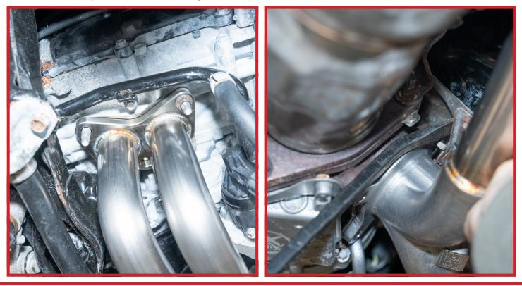
Because the supplied replacement turbo studs do not have Torx heads, use the best remaining OEM stud for the upper position and the new studs for the bottom two. Torque these studs to 11 ft/lbs. Ensure the upper stud passes through the heat shield.
