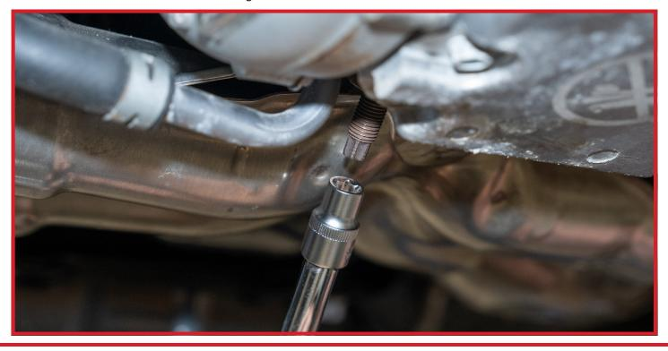
Remove the six 14mm nuts attaching the manifold to the heads. Leave one nut loosely threaded on each side to prevent the manifold from falling when removing the last nut. You will need to use an extension and reach in between the runners to get at the inner nut on each side.
