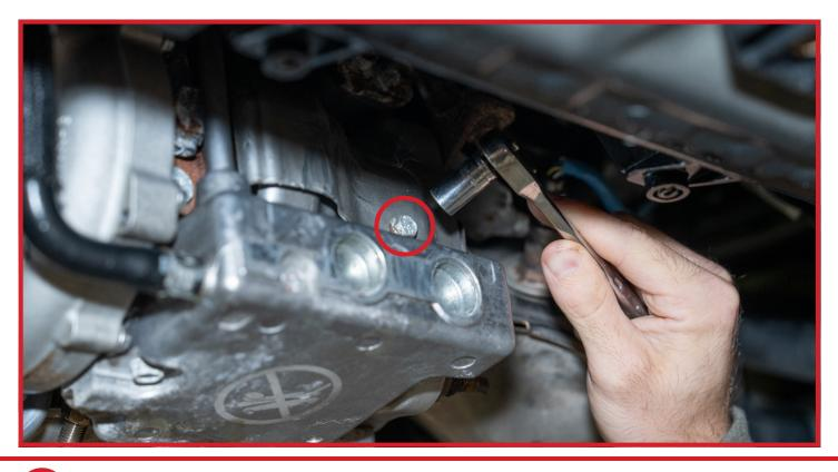
Use a deep 14mm socket to remove the three nuts holding the manifold to the turbo. Access the upper nut by maneuvering an extension between the oil pan and manifold.
