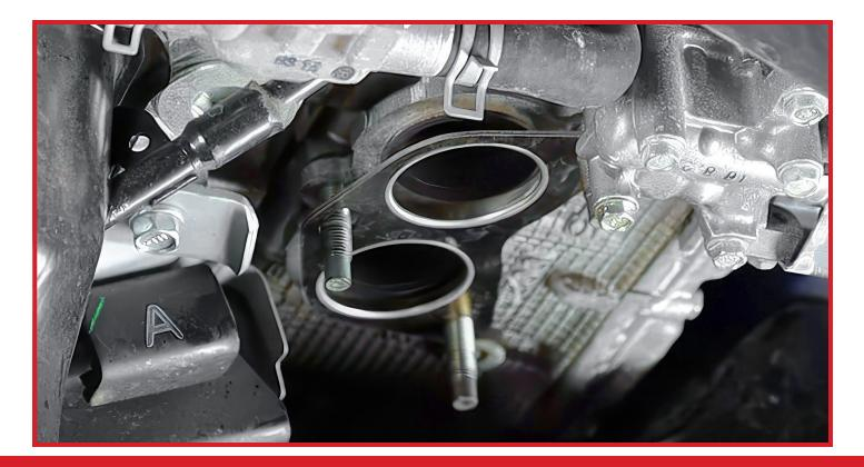
Take your Grimmspeed Header as well as the supplied turbo gasket and lift them up into place under the engine. Loosely install the included replacement nuts onto the studs in the heads, but do not fully tighten them yet. You may need to gently pry the turbo shield to get the header to seat in place on the turbo flange.
