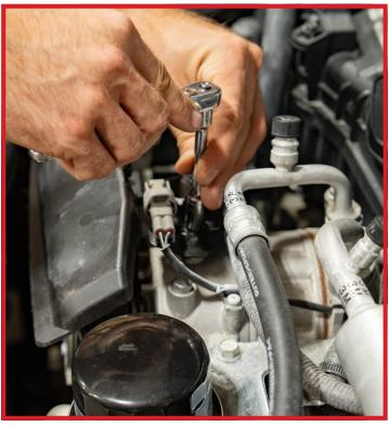
With the factory cover out of the way, you can now install the GrimmSpeed Pulley Cover Mounting Bracket included in your kit. Slip the bracket under the wiring connector for the AC Compressor and secure it in place with the two M6x12 bolts included in your Pulley Cover kit. Torque these bolts to 12 ft/lbs.
