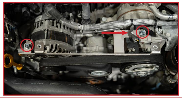
With the Mounting Bracket in place, rest your GrimmSpeed Pulley Cover over the bracket and align the mounting holes in the cover with the threaded inserts in the bracket. Using a 3mm allen wrench, Secure the Cover to the Bracket with the included M5 Bolts and GrimmSpeed Dress-Up Washers. Tighten these bolts down fully to 7.5 ft/lbs.
