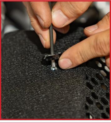
Once those two allen bolts are tightened, your Pulley Cover is installed. Reconnect your vehicle's battery and enjoy the upgraded aesthetics of your engine bay!
