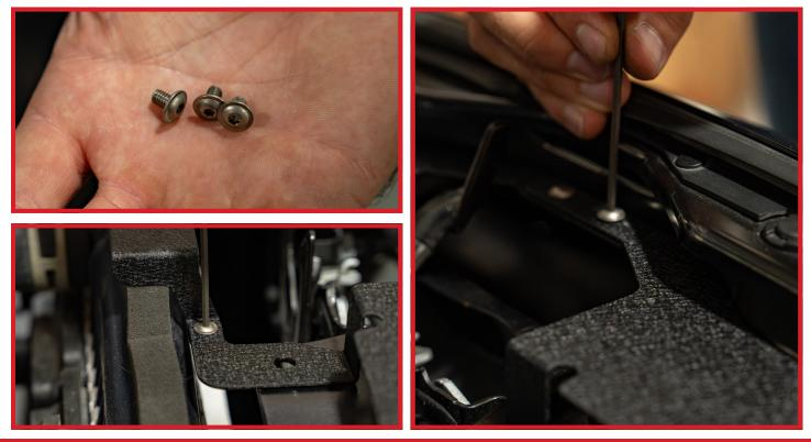
Grab the two larger Dressup Washers and their matching M6 bolts from your hardware kit and use them to secure the Radiator Shroud to the headlight mounting points as shown below using a 3mm allen key. Torque these bolts to no more than 12 ft/lbs.
