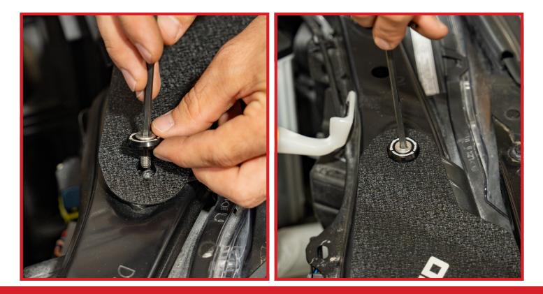
Secure the Radiator Shroud to the Mounting Bracket we added earlier with the last remaining smaller Dress-up Bolt/Washer combo. You can tighten this bolt to 7.5 ft/lbs. With the last of the Radiator Shroud hardware in place, you can fully tighten the three M4 bolts securing the two halves of the Radiator Shroud.
