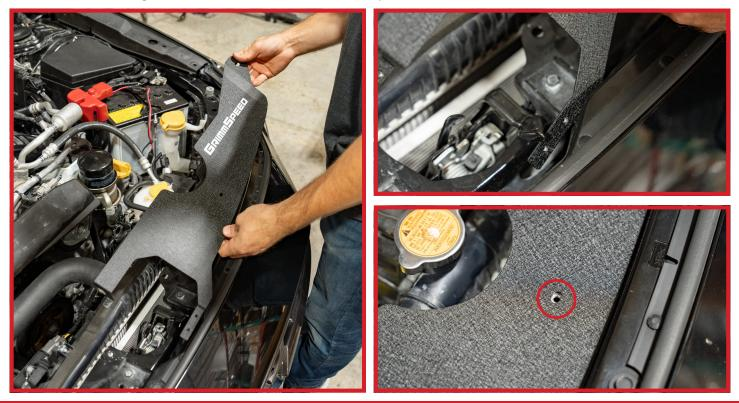
Before securing the driver's side of the Radiator Shroud into place, set the passenger's side of the Shroud in place as well. The small mounting holes where the two halves of the Shroud meet should line up as shown here.
