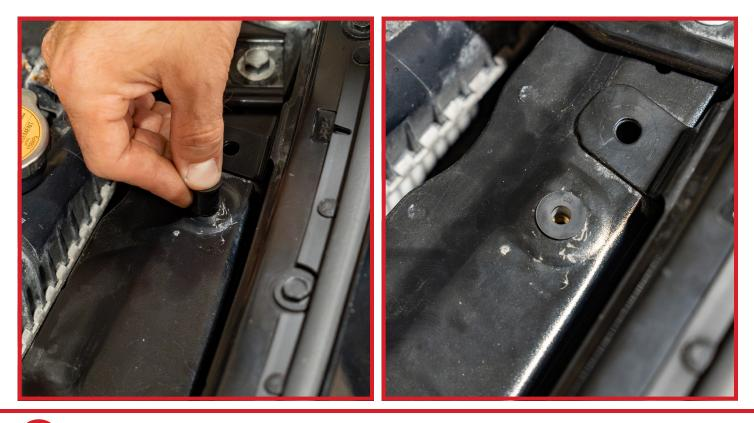
Grab the Radiator Support Mounting Bracket and the M6 Bolt included in your hardware kit and install them onto the radiator shroud as shown below. With a 10mm socket, tighten the bolt until it will not go any further to ensure that the rubber rivet nut is fully compressed and the bracket is securely mounted to the core support.
