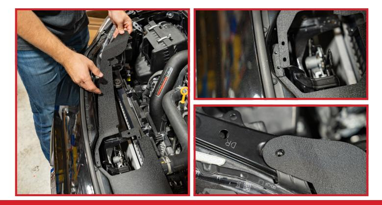
Grab the three small M4 screws included in your hardware kit and use them to bolt the two halves of the Radiator Shroud together using a 2.5mm allen key. These bolts are very easy to loose if they are dropped down into the radiator/fan assembly, so we suggest adding a dab of grease to the end of your allen key to stick to the bolt while installing. Leave these somewhat loose for now to allow for some adjustment.
