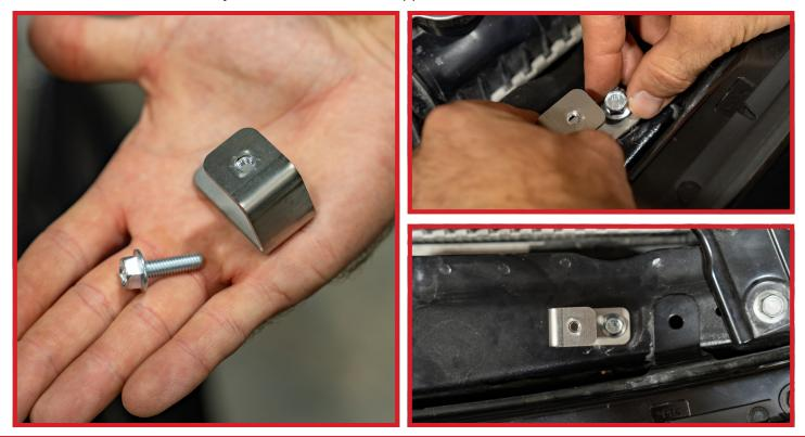
You can now begin installing the GrimmSpeed Radiator Shroud. Starting with the driver's side (the piece with the Logo), feed the front edge under the hood latch and lay the Shroud across the top of the radiator. The middle mounting hole should line up with the threaded insert on the mounting bracket we installed in the last step.
