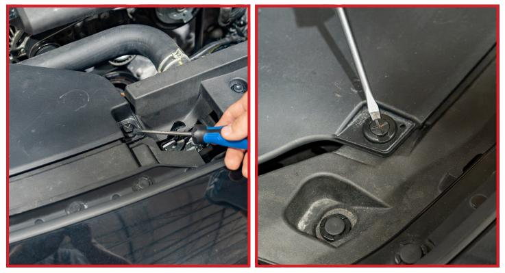
With the intake duct out of the way, we can work on removing the factory radiator shroud. There are 3 more plastic pop clips across the shroud that hold it in place. You will also need to remove the two 10mm bolts securing the headlight mounting tabs to the core support. Once all of the hardware is removed, you can remove the factory cover.
