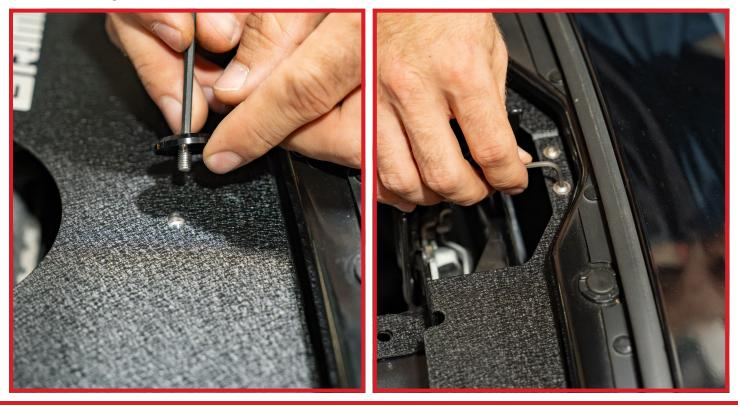
The last step is to reinstall the factory intake duct into the engine bay vy inserting it in to the opening in the air box and securing it to the GrimmSpeed Radiator Shroud using the two plastic pop clips we removed at the beginning of this install.
