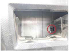
Find the black bracket and plastic push clip. Install the bracket from under the car with the prongs facing down and the bracket going on the outside of the plastic cubby, on both sides. So the pass side of the bracket is sitting on the outside of the j-nut and the other on the outside as well. Then install black push clip into the driver side hole.
