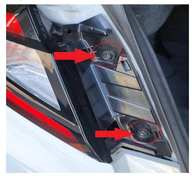
After removing the 2 8mm Screws using two hands pull the tail light towards you. It is clipped in on the outside corner with a While Male Push clip and no other screws. You will now see the OEM harness that connects to the Tail Light.
