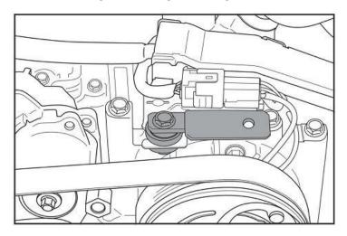
D) Align the Large and Small Bracket as shown in the image below so that they are aligned with the pulley
