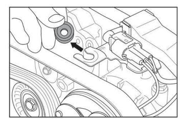
B) Prepare the SHORT bracket, LONG screw, 2 x WASHERS and LOCK NUT as shown in the image below. Using 10mm Socket and 10mm Wrench tighten the LOCK NUT and SCREW so it leaving ¼" space between washers.
